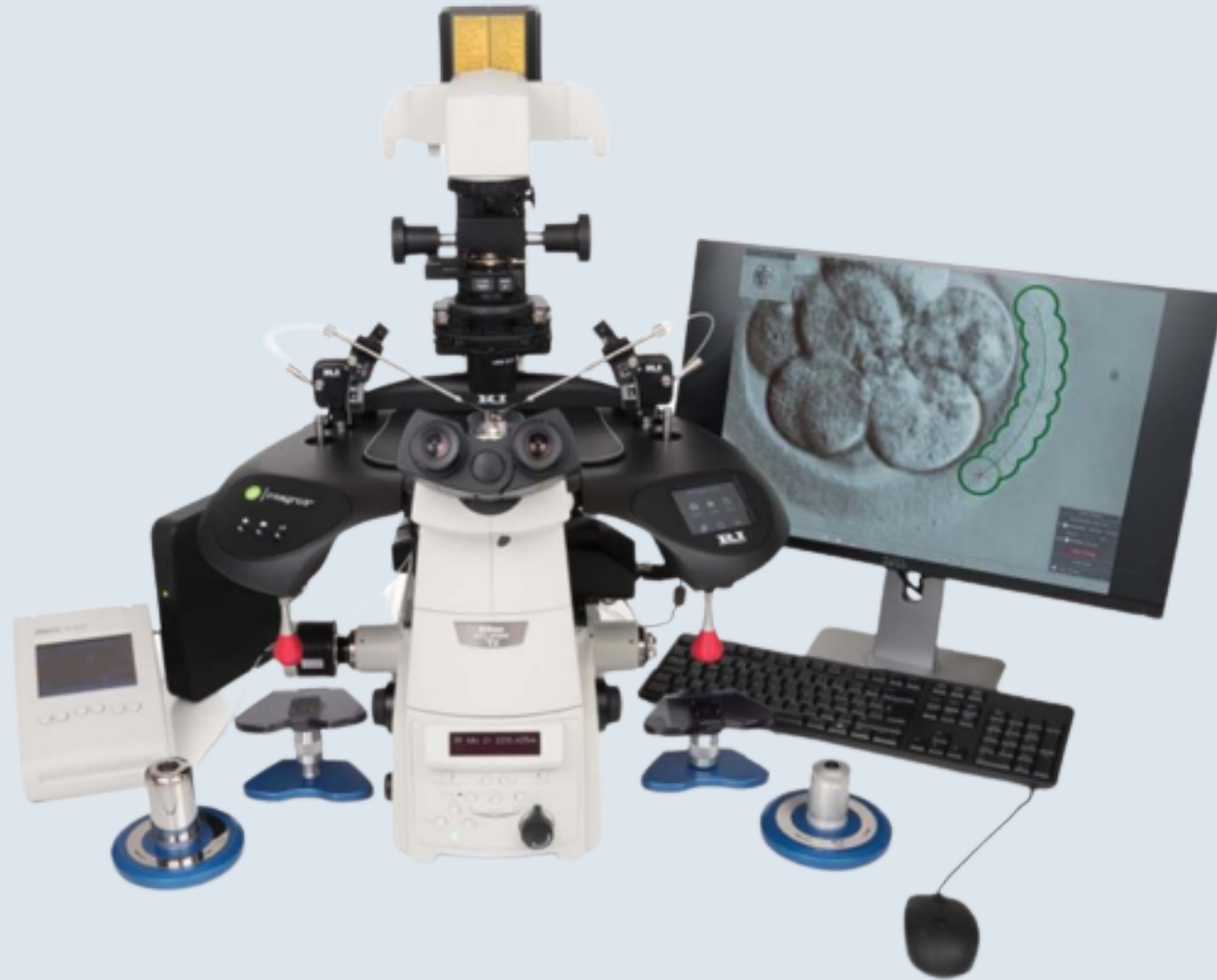
RI Integra 3 Micro-manipulator with Nikon Inverted Research Microscope (Ti2-U)
